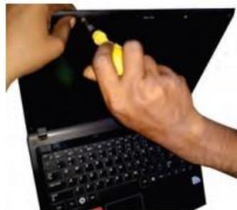
**Fig. 2.22: Remove the four screws securing LCD screen**
