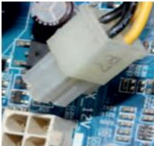
**Fig. 1.45: unplug 4-pins AUX power connector from power connector from motherboard**
