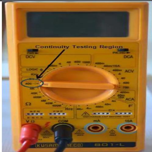
**Fig. 3.16: Continuity Test using Multi meter**
