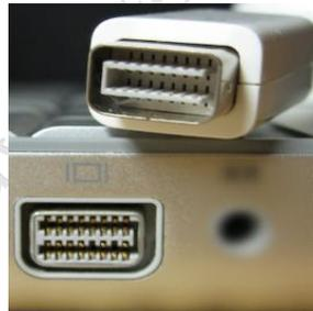
**Fig. 1.38 Mini-DVI port and its compatible cable**
