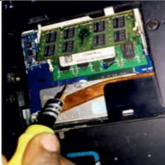
**Fig. 2.11: Remove RAM memory modules**
