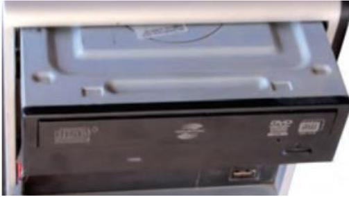
**Fig. 1.14: Insert optical drive**
