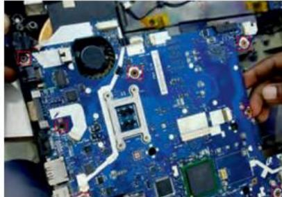
**Fig. 2.18: Disconnect cable from motherboard and remove screws**
