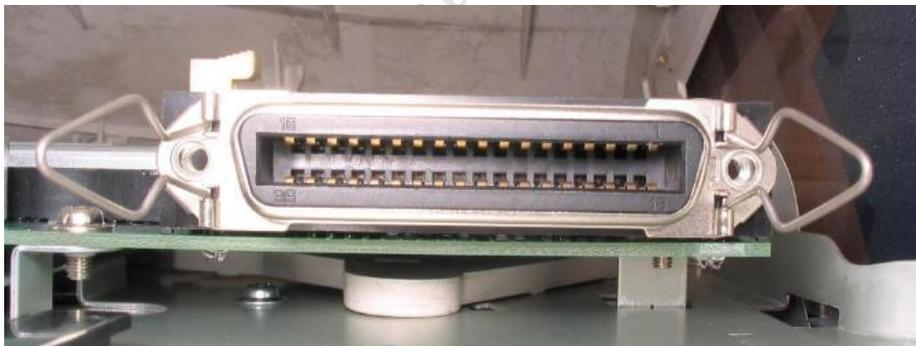
**Fig. 1.31 36 pin Centronics port**
