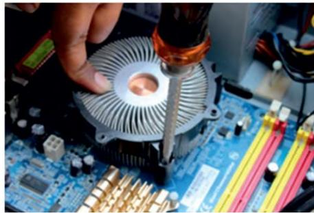
**Fig. 2.12 Screwing the heat sink**
