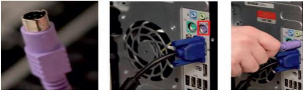
**Fig. 1.23: Connecting keyboard in PS/2 port**
