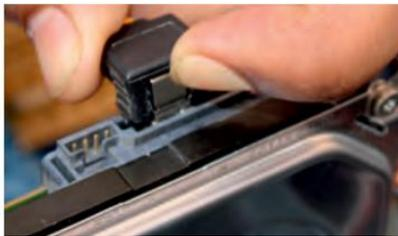
**Fig. 1.16: Connect cable IN to HDD**
