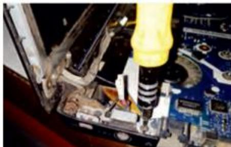
**Fig. 2.16: DC power jack mounted under display hinge**
