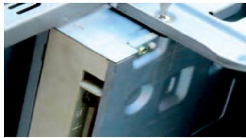
**Fig. 1.15: Tighten screws of optical drive**
