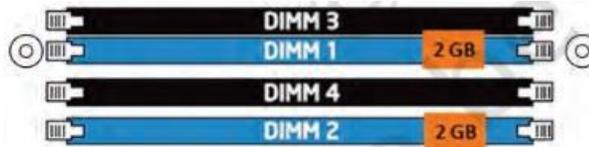
**Fig. 3.8: Dual-channel with two DIMMs**
