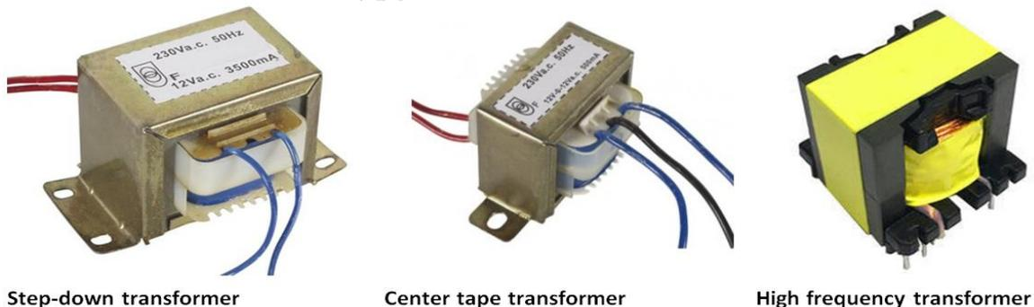
**Fig. 1.24 Different types of transformer**
