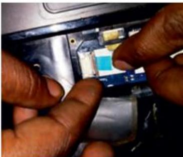
**Fig. 2.20: Keyboard permanently attached to top case**
