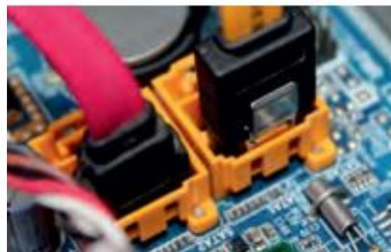
**Fig. 1.46: Unplug SATA cables from motherboard**
