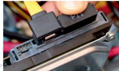
**Fig. 1.17: Press cable socket for proper connection**
