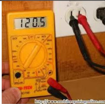
**Fig. 3.12: Measurements of AC Voltage**
