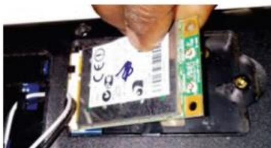
**Fig. 2.17: Disconnect Wi-Fi Module**
