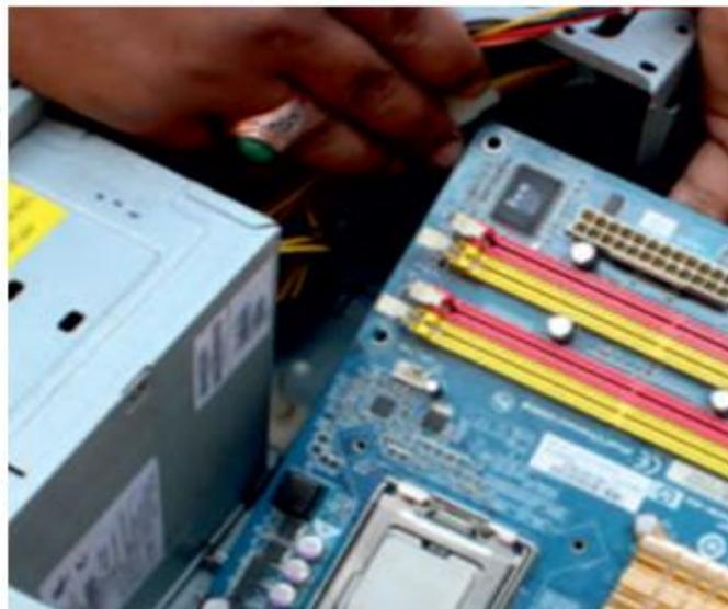
**Fig. 1.54: Removing the motherboard**
