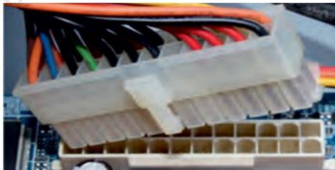
**Fig. 1.18: Plug-in 20-pin ATX power connector to motherboard**
