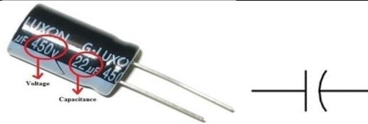
**Fig. 1.18 (a) Capacitor (b) Capacitor Symbol**
