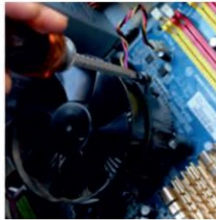
**Fig. 1.42: Remove the system fan**
