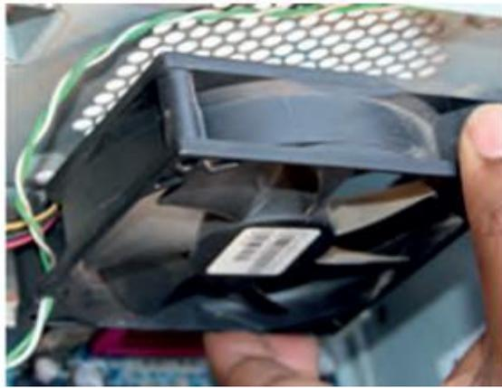
**Fig. 1.41: Unscrew fan**
