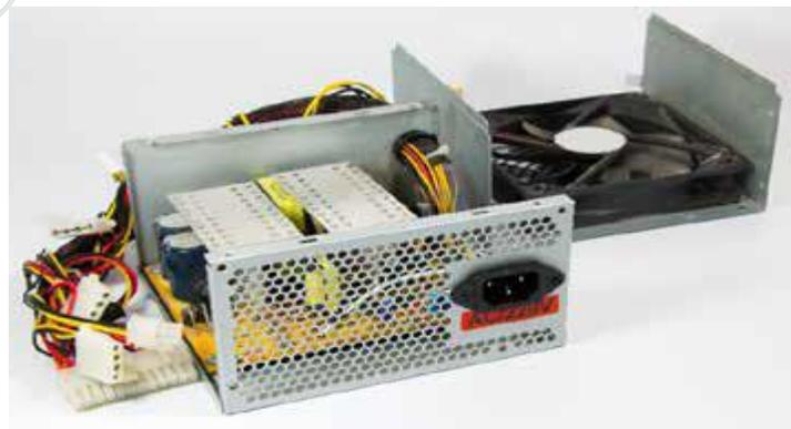
**Fig. 2.12 Interior view of a PSU**
