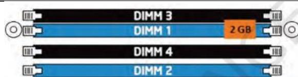
**Fig. 3.7: Single-channel with one DIMM**
