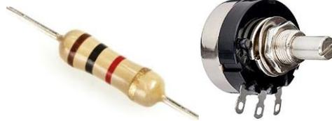
Fig.1.17 (a) Fixed resistor
