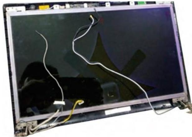
**Fig. 2.24: Separate LCD screen from back cover**
