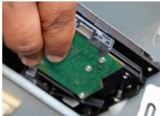
**Fig. 1.51: Remove HDD**
