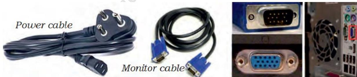
Fig. 1.21: Display cable and ports
