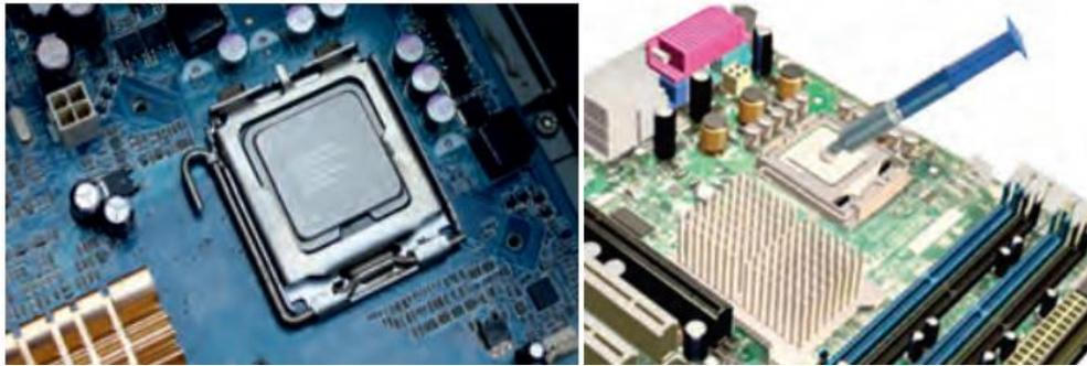
**Fig. 2.9 Installing CPU on the motherboard**      **Fig. 2.10 Applying thermal compound on CPU**
