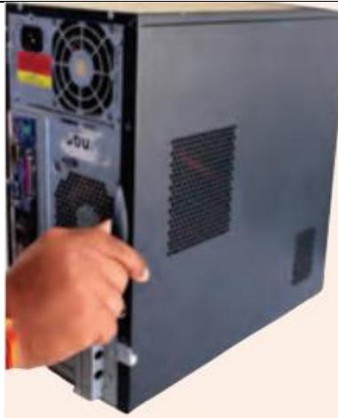
**Fig. 1.10 Remove the side panel**
