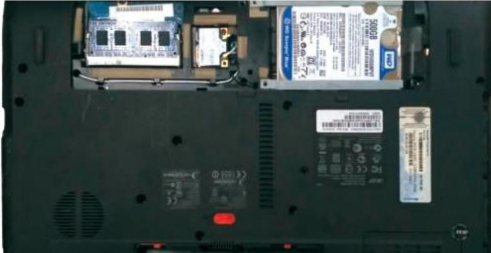
**Fig. 2.1: Back panel of a laptop**
