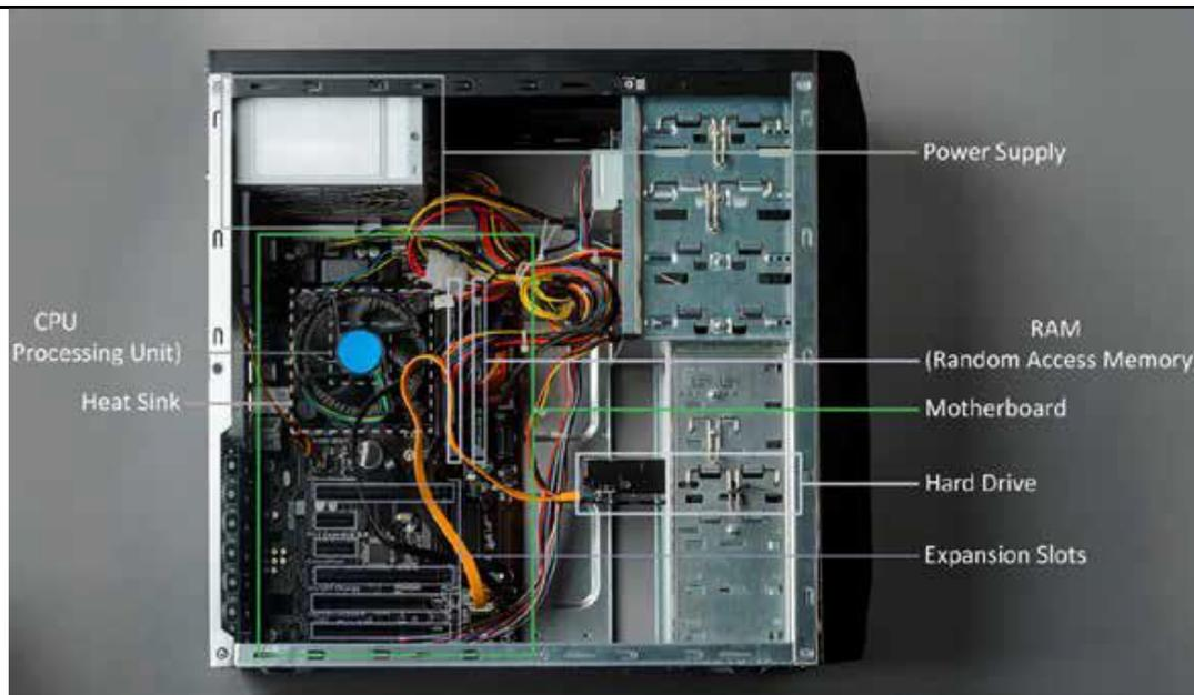
**Fig. 2.13 Internal hardware components**
