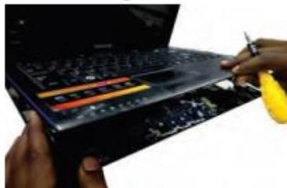
**Fig. 2.6: Separate palm rest from bottom case**
