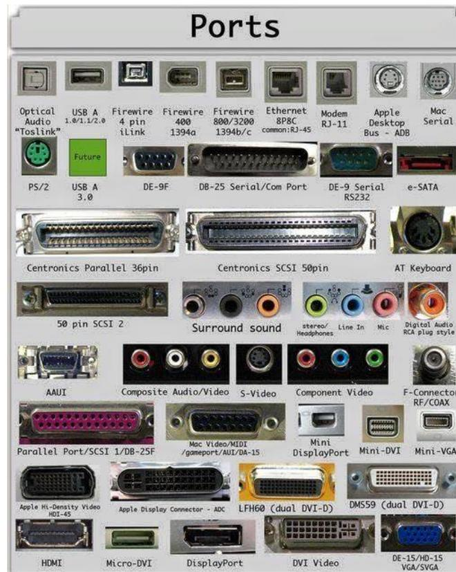
**Fig. 1.26 Input Output Ports and System Resources**
