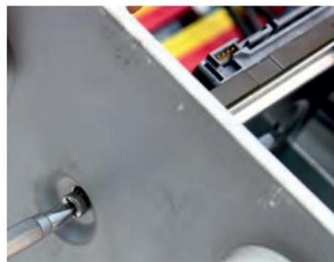
**Fig. 1.13: Tighten screw of HDD**
