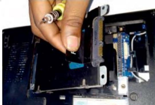
**Fig. 2.9: Remove hard drive assembly    Fig. 2.10: Disconnect SATA cable**
