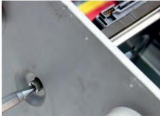
**Fig. 1.50: Unscrewing of HDD**
